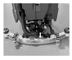
Step.5: Check the suction rake strip and make appropriate adjustment (see "Suction Rake Strip Adjustment")
