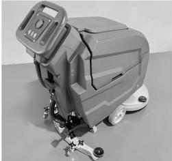
Step.3: For different floor cleaning requirements, the water output can be controlled by adjusting the water valve switch up and down.
