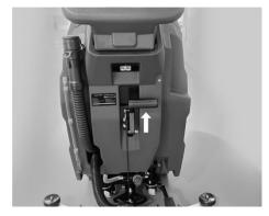
Step.3: Mount the suction rake onto the suction rake mounting bracket, as shown in the figure . Be sure to fully place the fastening knob in the slot and then tighten the knob.
