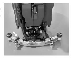
Step.4: Connect the suction pipe to the suction rake assembly, as shown in the figure.
