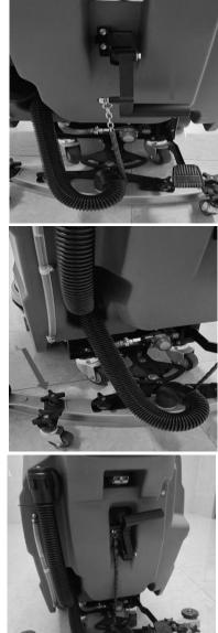
Step.2: Press down the brush disc lifting pedal and move it to the right (as shown by the arrow) so as to raise the brush disc motor.
