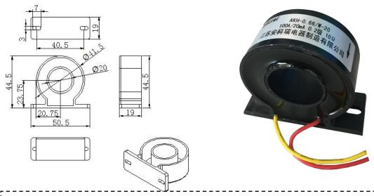
Noted: Primary current flows from P1 to P2(glue-pouring), secondary outlet line is fixed to P2 side, the red line is S1, the yellow line is S2, the line length is 2m.
