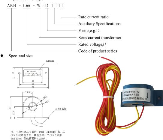
Note: Primary current flow from P1 to P2(Glue surface). The yellow second wiring is S2, the red is S1. The outlet length is 2m + 10cm.
