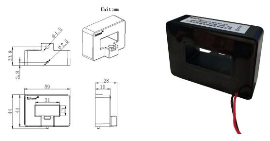
Note: Primary current flow from P1 to P2(Glue surface). The black second wiring is S2, the red is S1.
