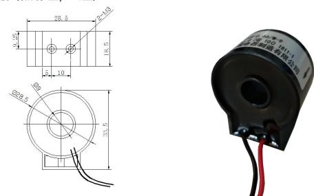
Note: The primary current enters from P1 and exits from P2 (glue filling surface). The red and black lead lines are S1 and S2. The length of the lead line is  $2m\pm10$ cm.
