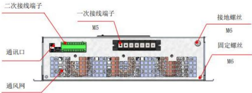
Figure 3-29 Top of 30A wall-mounted module
