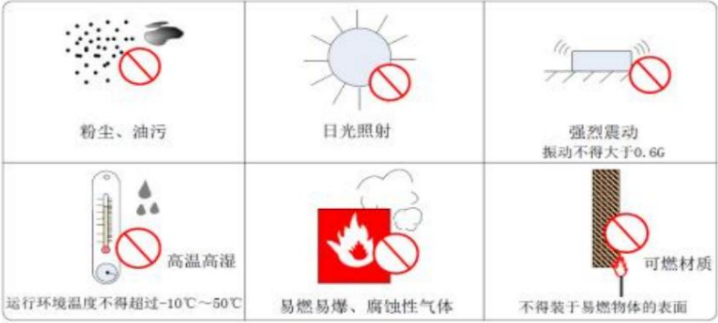
Figure 5-1 Schematic diagram of installation environment requirements
