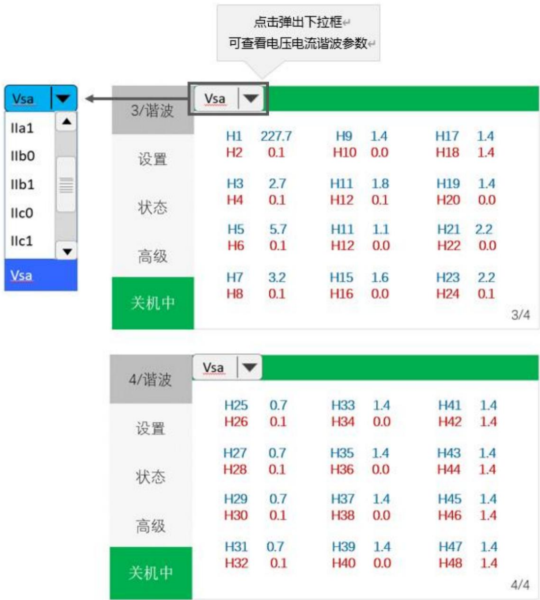
Figure 8-4 Monitoring interface - harmonic parameter interface
