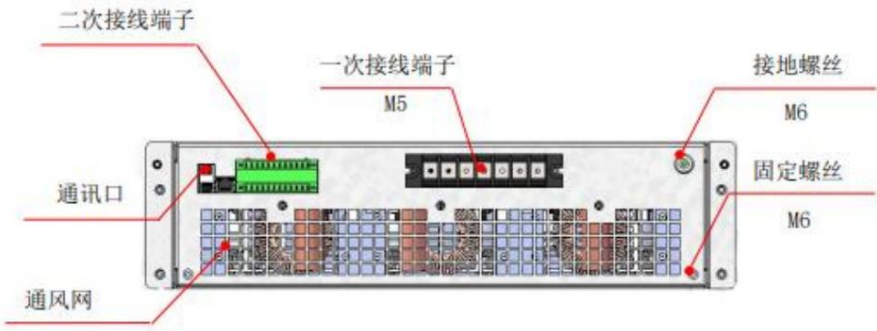
Figure 3-25 Back of 30A drawer module
