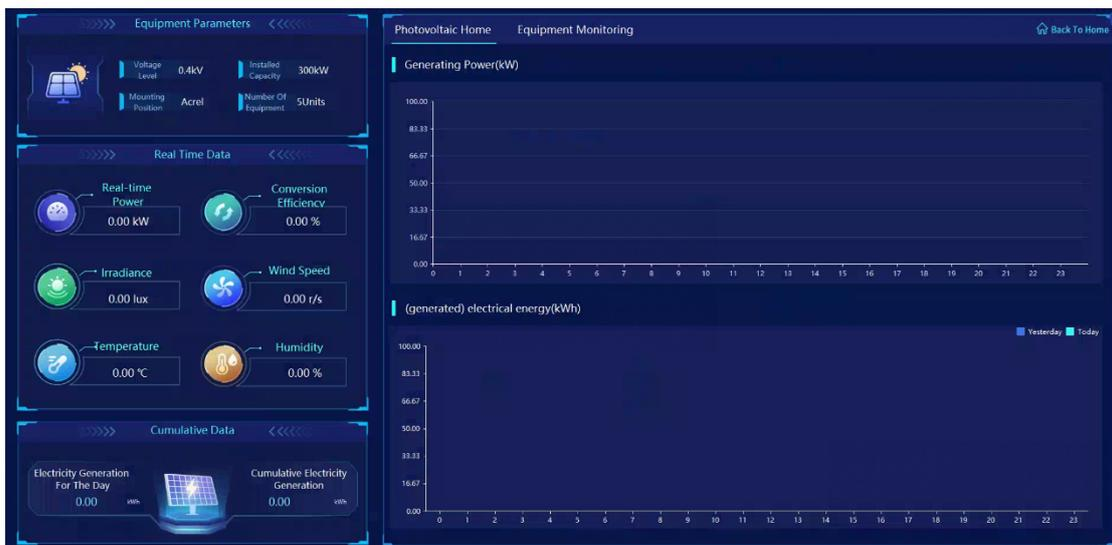
Fig. 3.10 Main Monitoring Interface of PV Power System
