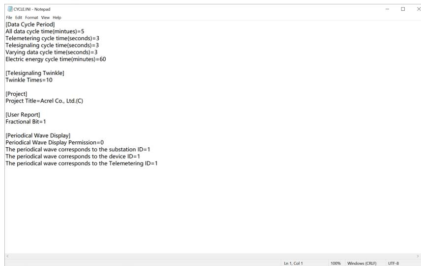
Fig. 4.12 Remote message blinking times profile content
