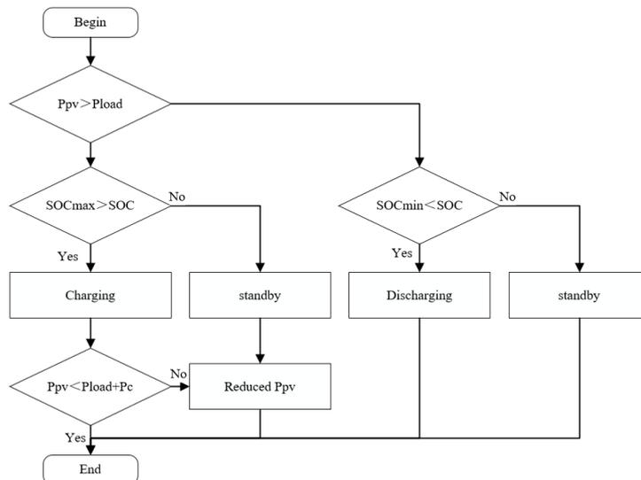
Fig. 3.23 Logical Control Flow of On-grid Running Mode
