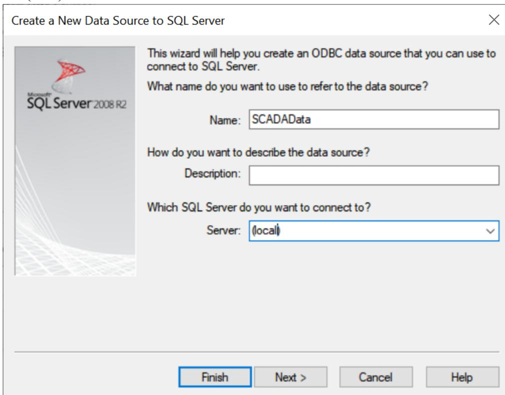
Fig. 4.5 Enter the data source Name and connected Server
