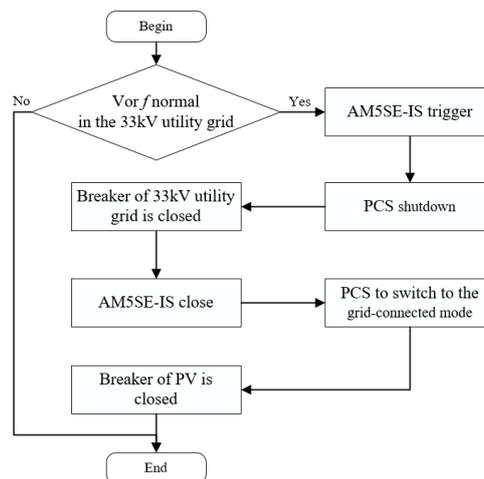
Fig. 3.25 Logical Control Flow of Grid-islanded Running Mode
