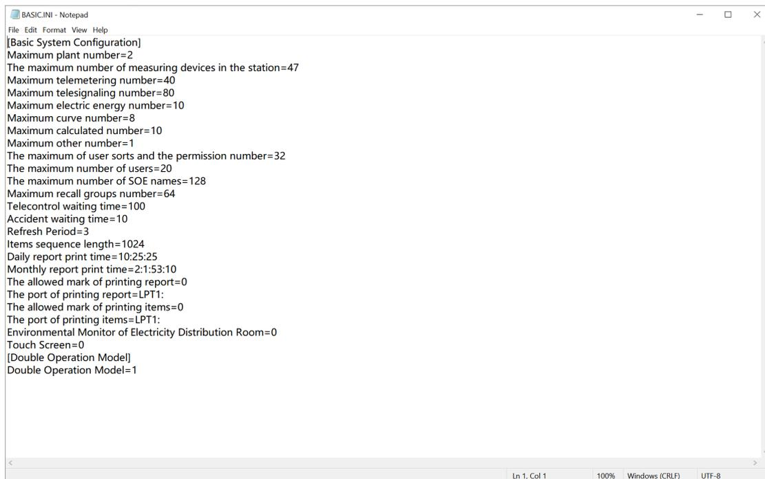
Fig. 4.11 Basic system configuration
