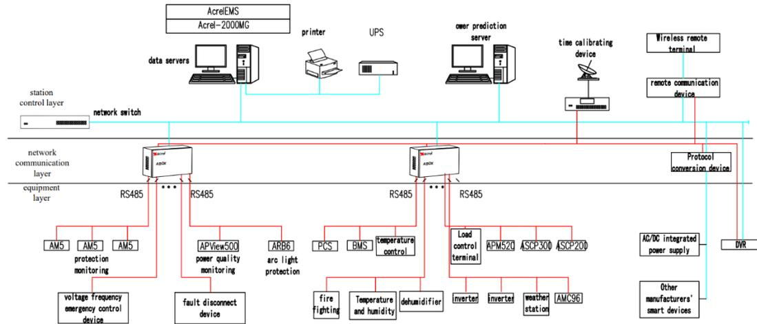
Fig. 2.1 Typical Networking of Microgrid Energy Management System
