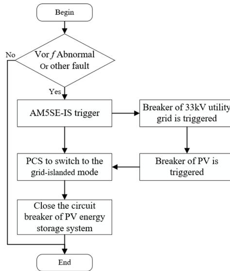
Fig. 3.24 Logical Control Flow of Grid-islanded Running Mode
