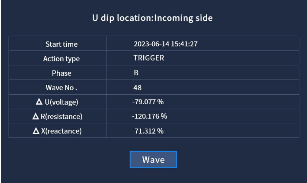
Fig. 4.27(a) Voltage dip location:incoming side
