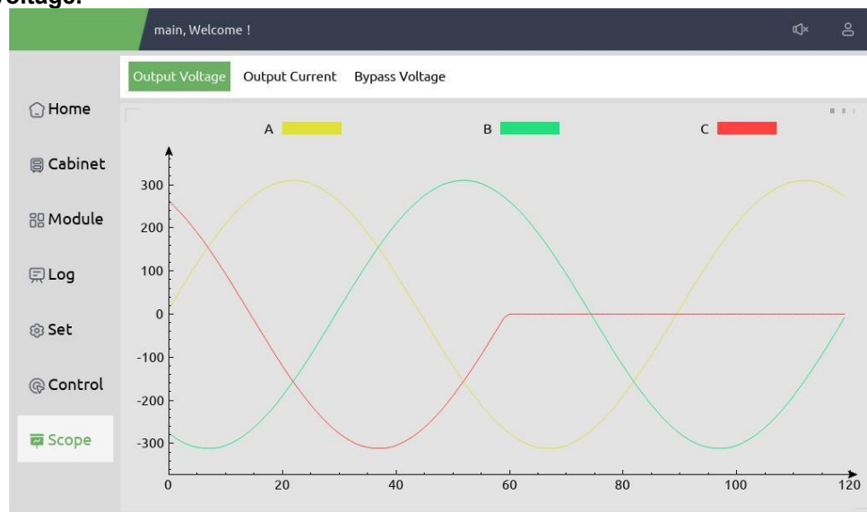
Fig.7-9: output and bypass waveform
