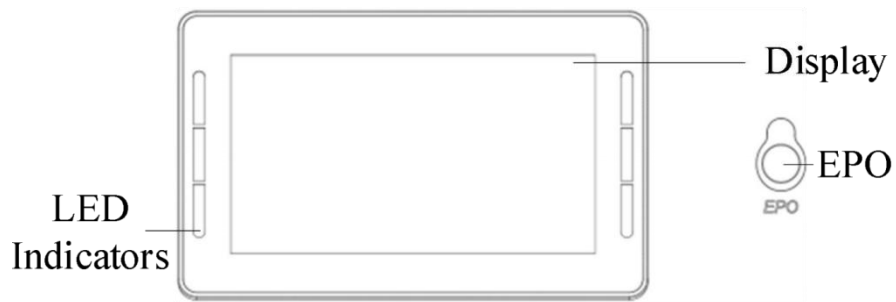
Fig.7- 1: UPS operator control and display panel
