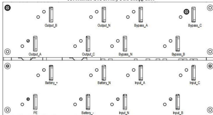
Figure 1-5-2 4-module cabinet and 6-module cabinet terminal block layout diagram
