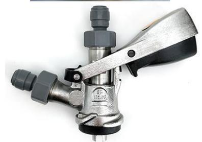
Once you have matched the correct keg coupler to the keg you will need to set up the commercial keg coupler. On a keg coupler there is an inlet for gas and an outlet for liquid. The gas inlet is positioned on a 45-degree angle and the liquid outlet is positioned vertically. It is important to connect the gas line and beer line to the correct inlet and outlet. This is described in the image below.
