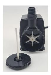
**Step 4.** Pull the impeller out of the impeller cavity. Be careful when removing the impeller as the magnet is quite strong and may snap back into place quickly with a lot of force.
