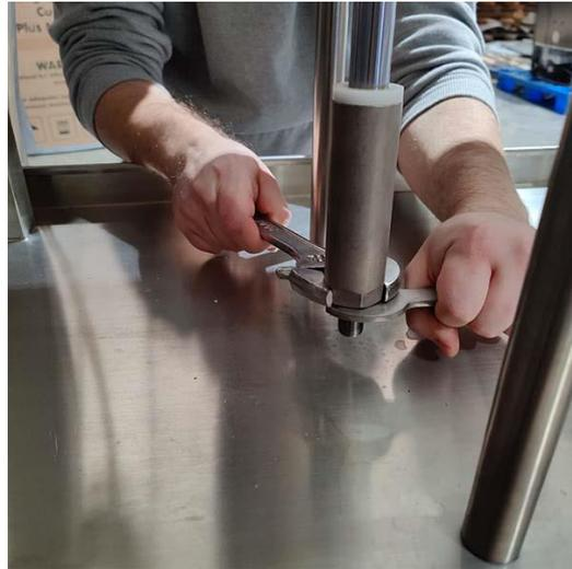
**2.6.4** – Rotate the bump stop shaft further down with your hand. Its best to go further down than you need.
