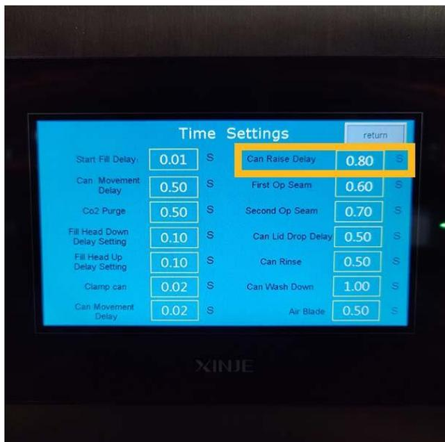
*If you are not familiar with the functions of these Timers, it is best to take note of the default values and adjust the setting you're not familiar with up by to 10 seconds and run a can through. This will then help you get a better understanding of what that timer function does.*
