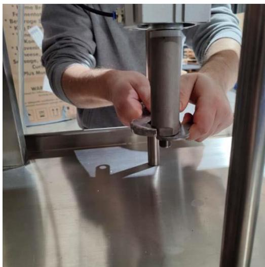
**2.6.6** – Once the can feels firm and in place, rotate the Bump Stop Shaft upwards until it touches the piston block. Followed by the locking nut. Then use the two spanners again to tighten against each other.
