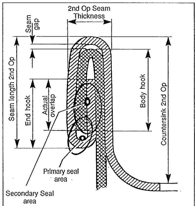
The forming of the 1<sup>st</sup> operation seam is the most important operation as this operation takes the end curl and can flange and begins the forming process. It's the formation/dimension of this 1<sup>st</sup> seam that controls the effectiveness of the 2<sup>nd</sup> operation seaming roll profile in achieving a hermetic seal.
