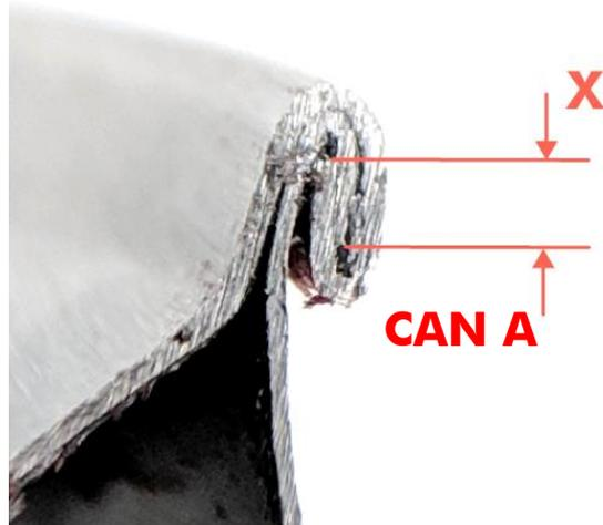
This measurement should be at least 0.4mm however if this measurement is over 1mm it is ideal.
