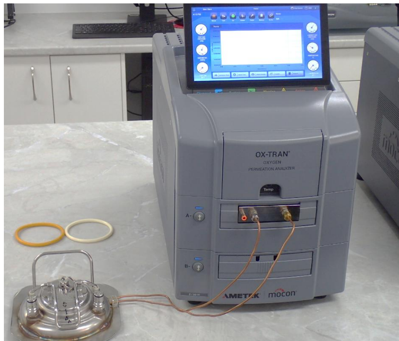
Photograph of keg-top connected to Ox-Tran 2/22 test instrument.
