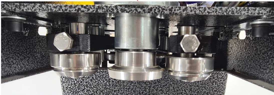
1st and 2nd Operation Rollers in Furthest Position from Chuck (Middle)
