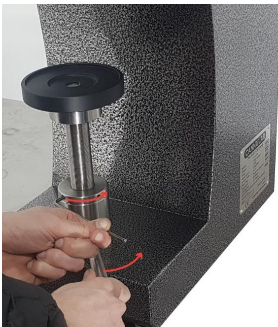
Left: Loosening coupling nut
