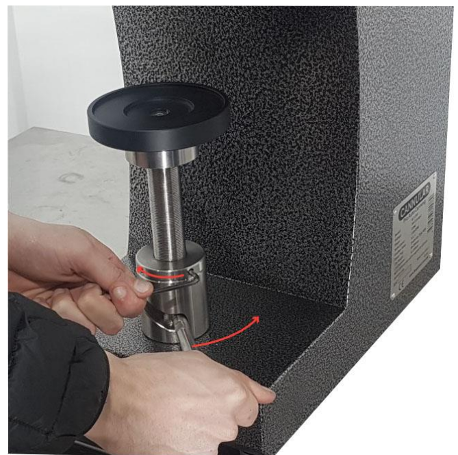
Right: Tightening coupling nut
