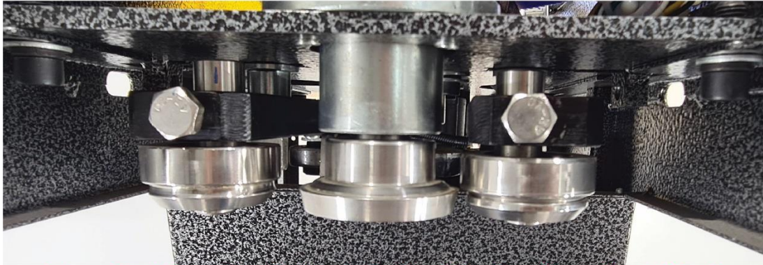
1st and 2nd Operation Rollers in Furthest Position from Chuck (Start)
