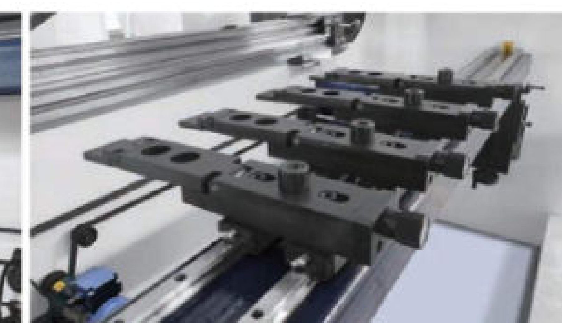
双直线导轨横梁和多挡指结构 Double linear guide beam and multi-stop finger structure
