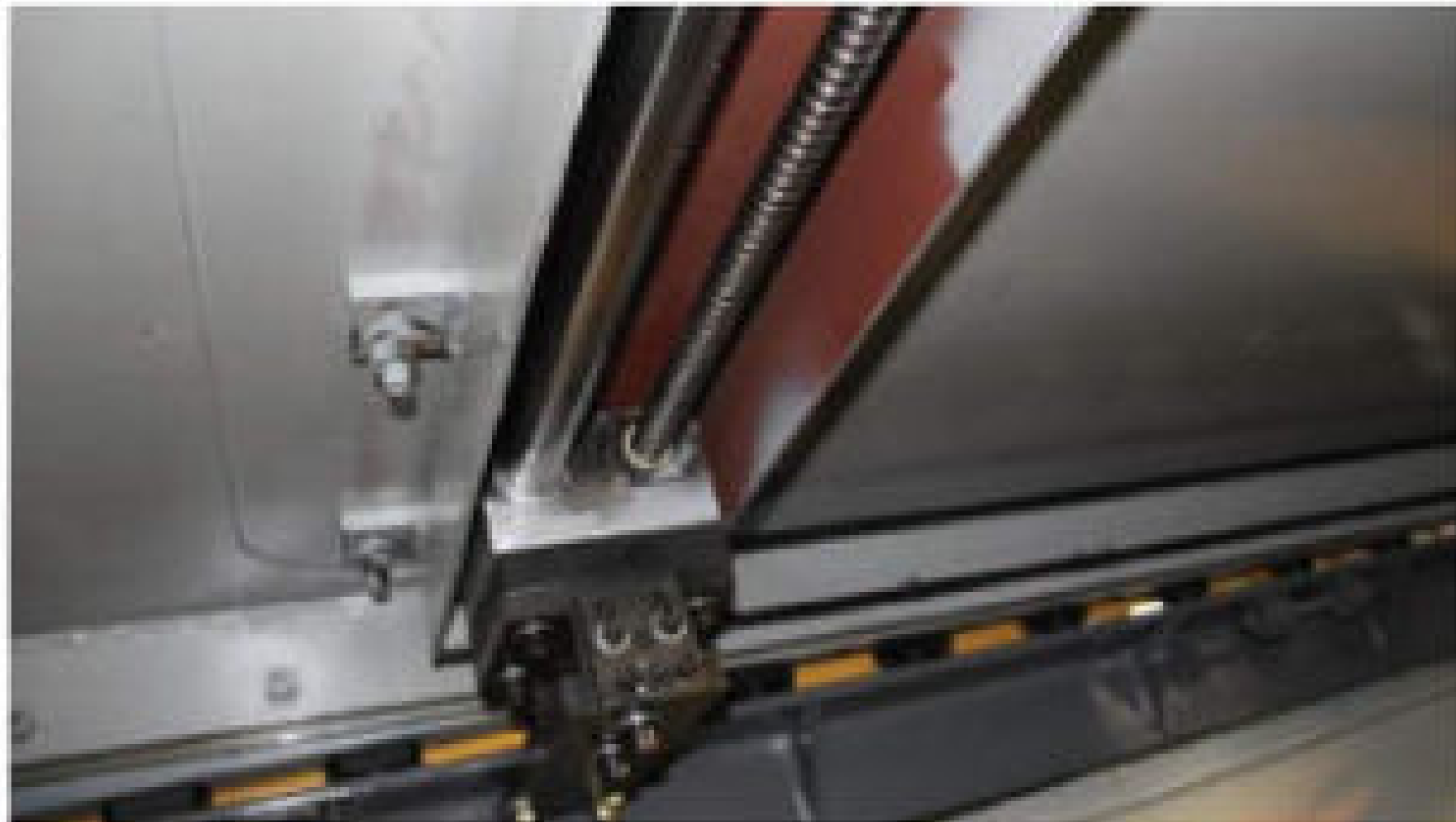
X轴滚珠丝杆和研磨光杆 X axis ball screw and polished rod
