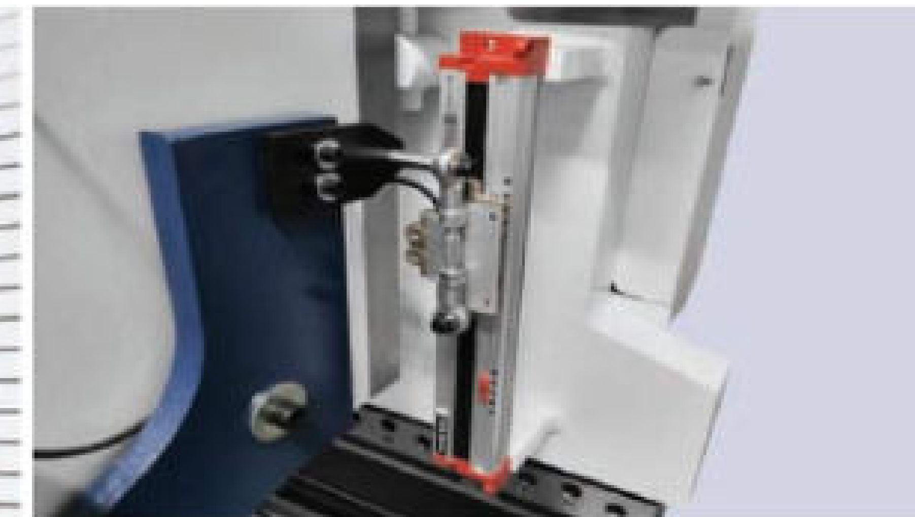
磁栅精准检测定位 Magnetic grid accurate detection and positioning
