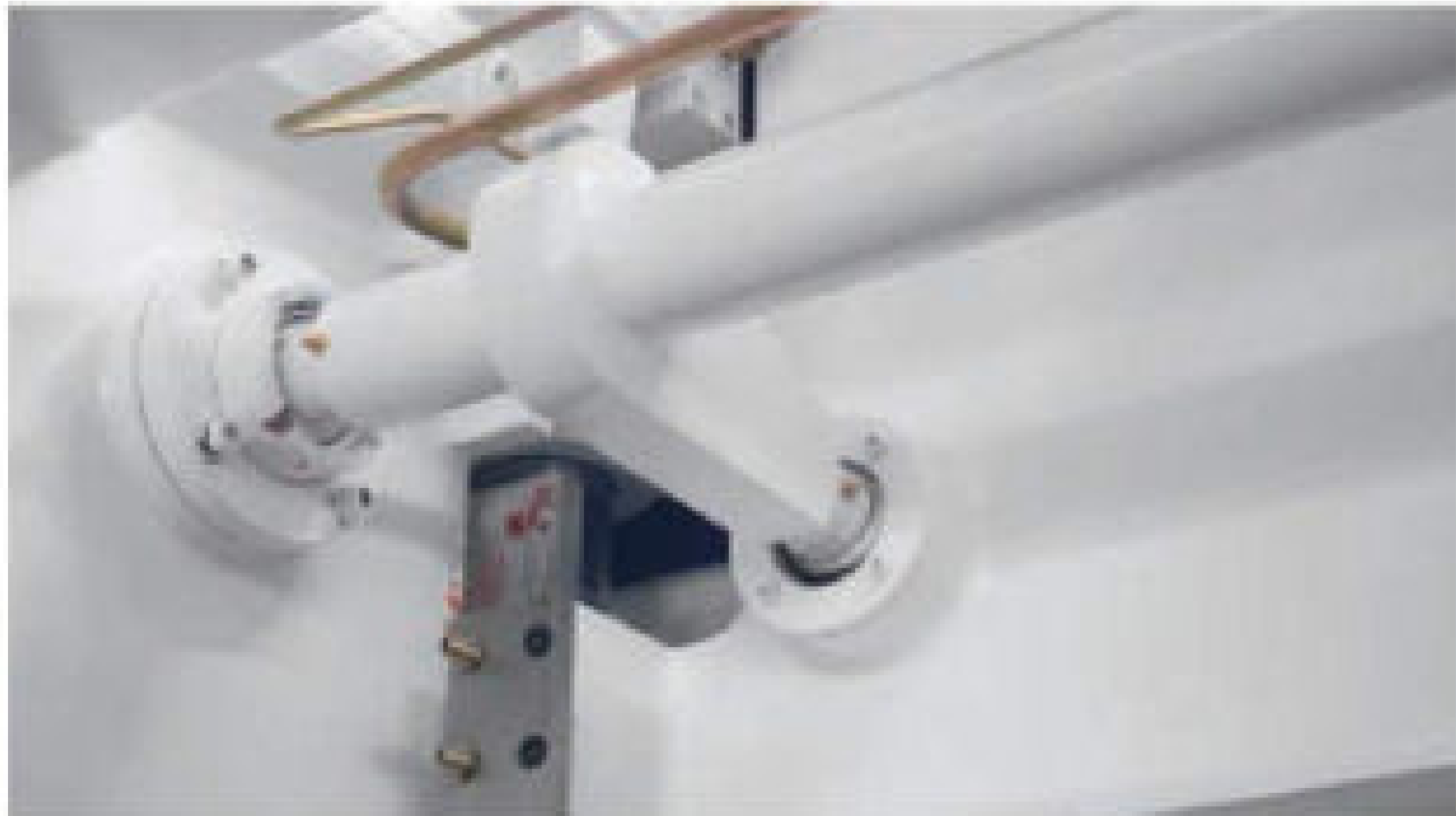
扭轴同步结构 Torsion axis synchronous structure
