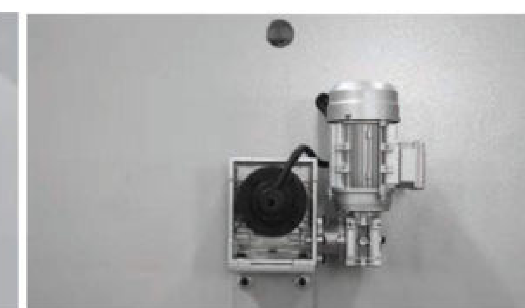
电动调节刀片间隙 Electric adjustment of blade clearance
