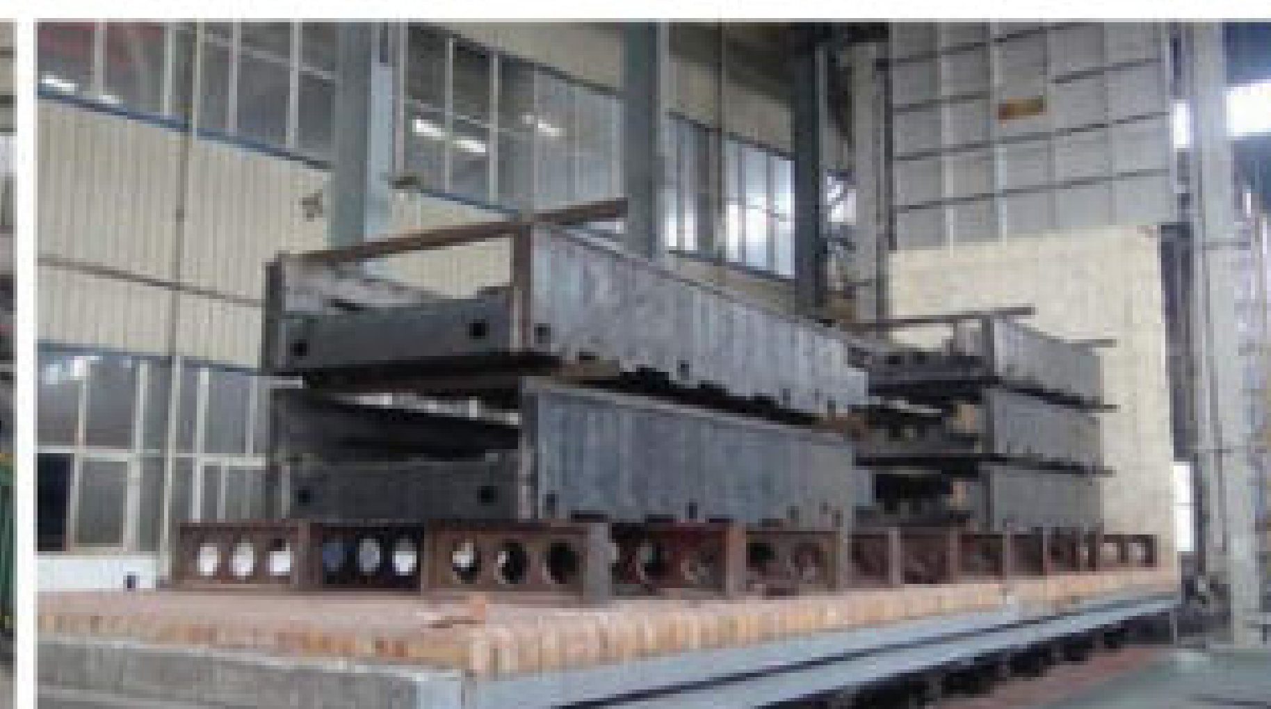
床身整体退火 Whole bed annealed
