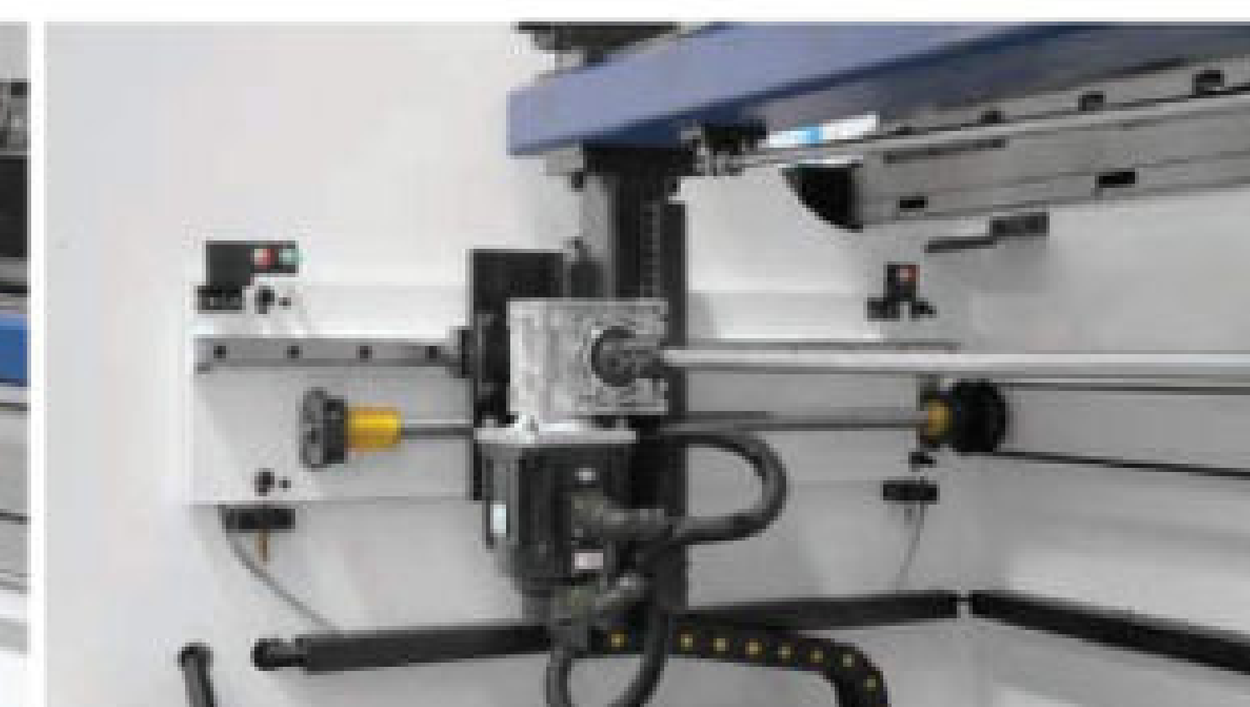
R轴齿轮同步 R axis gear synchronization
