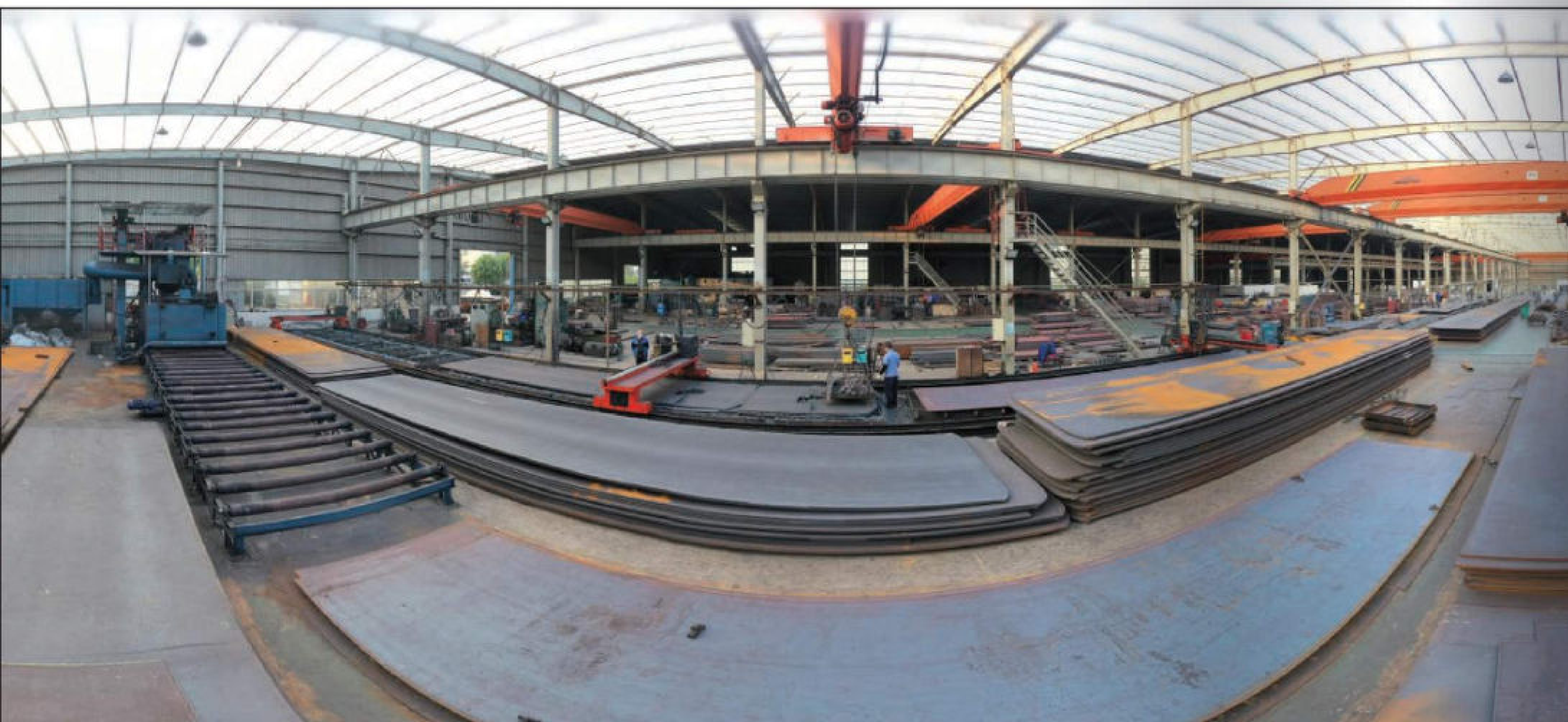
下料车间, 抛丸、切割生产线 Cutting workshop, shot blasting and cutting production line
