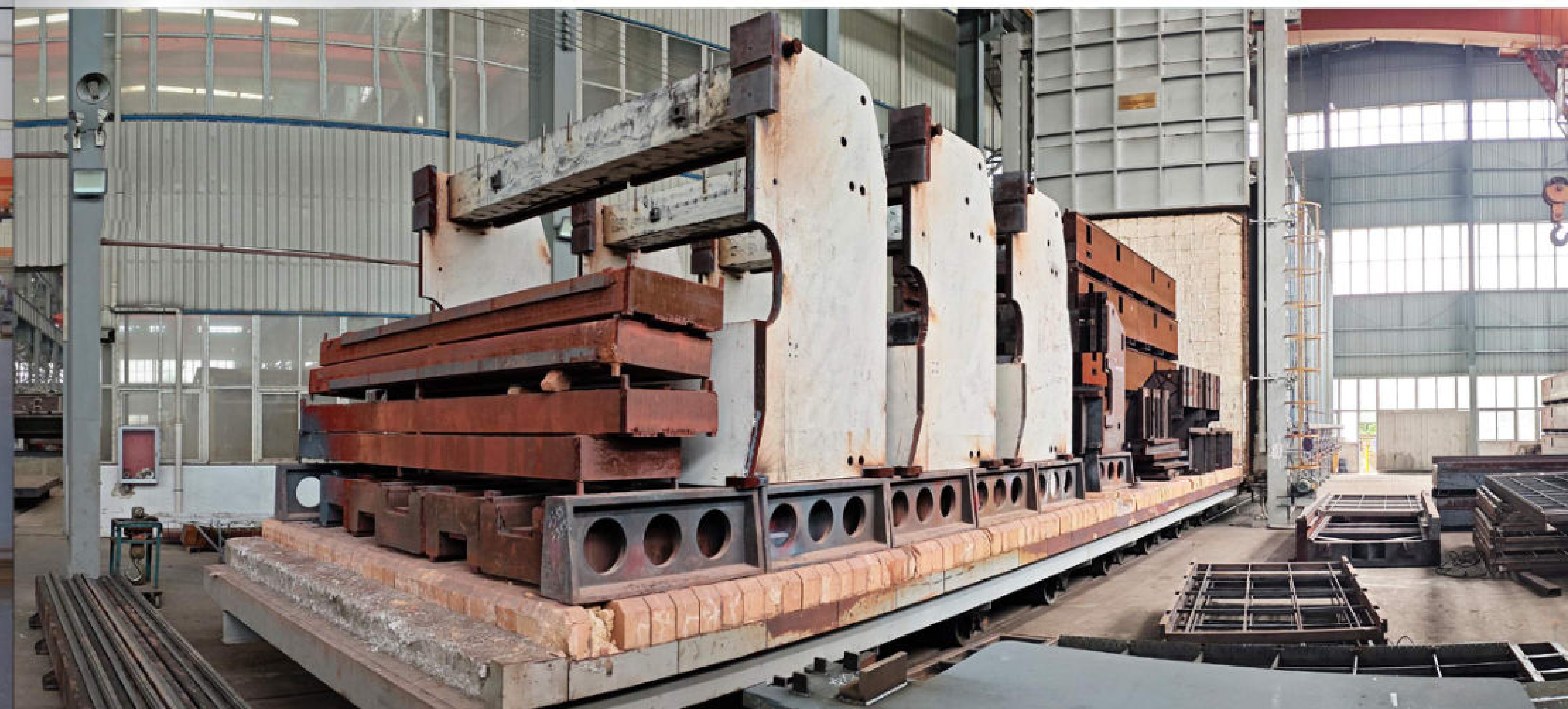
燃气台车式热处理炉 14m*4m*4.6m Gas trolley type heat treatment furnace 14m ×4m ×4.6m
