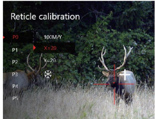
3. Adjust the X-axis and Y-axis using the scroll wheel to align with the point of impact.
