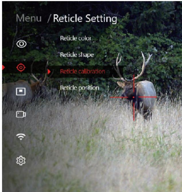
2. The red reticle remains fixed at the center of the screen. The white reticle represents the currently adjusted reticle. When entering this option for the first time, the white and red reticles coincide ( $X=0, Y=0$ ), indicating the current coordinate values of the reticle. "100M" represents the adjustable distance of the point of impact.
