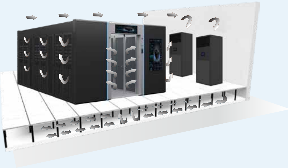
Room-level Cooling Airflow
