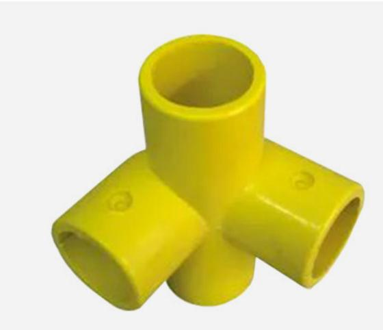
The GRP 116 Mid Corner is a 90° corner joint, often used in a GRP handrail or guardrail to continue the middle rail on a 90° corner, but can also be used to build rectangular or square structures. The upright passes vertically through the GRP fitting. Often used with the GRP-128 Top Corner.
