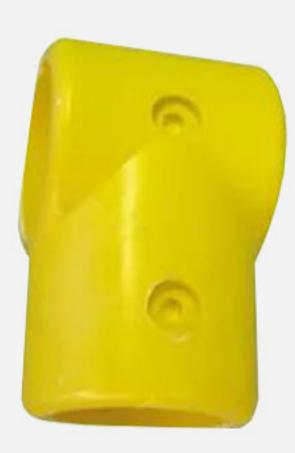
The GRP 101 Short Tee is a 90° tee connection, typically used in a GRP handrail to connect vertical posts to the top rail, or to join the midrail to the end post. The tube cannot be joined within the top of the fitting – the GRP-104 Long Tee can be used as an alternative if this is required.
