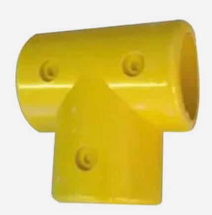
The GRP 104 Long Tee is a 90° tee connection, typically used to connect vertical posts to the top rail of a GRP handrail. The GRP-104 can be used where two lengths of tube need to be joined within the top of the fitting.
